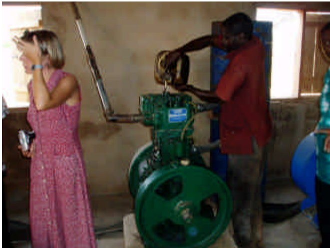
Figure 2 : Jatropha biodiesel being used to power a stationary engine.
